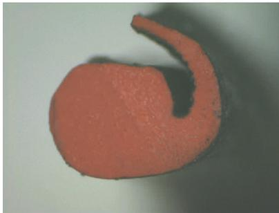
Example of Gross Extrusion Cross Section
