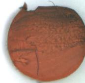
Example of Cross Section of Extrusion Failure
