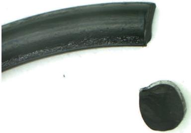
Example of extrusion and wear
