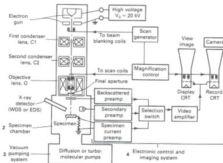
FIGURE 1: Basic components of the scanning electron microscope - WDS, wavelength-dispersive spectrometer; EDS, energy-dispersive spectrometer; CRT, cathode-ray tube
