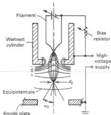
**FIGURE 2:** Conventional tungsten hairpin filament electron gun
