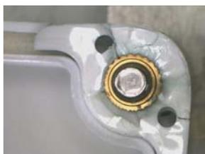
Cracking at an insert poly-carbonate piece
